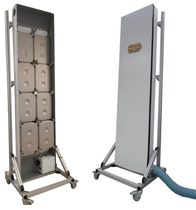
Picture 3: E2VENT Latent Heat Thermal Energy Storage prototype
